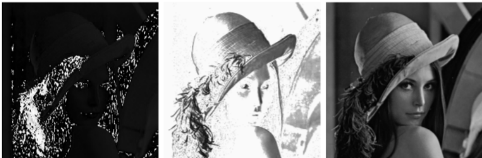
FIGURE 7.37 HSI components of the RGB color image in Fig. 7.36(a). (a) Hue. (b) Saturation. (c) Intensity.
