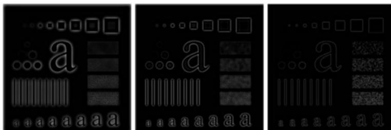
Results of highpass filtering the image in Fig. 4.41(a) using a BHPF of order 2 with  $D_0 = 30, 60, \text{ and } 160$ .
