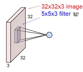
**Result:** dot product between the filter and a small  $5 \times 5 \times 3$  chunk of the image.
