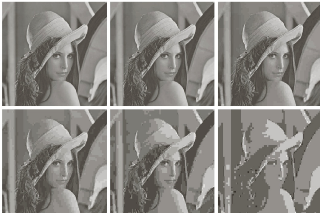
FIGURE 8.31 Approximations of Fig. 8.9(a) using the DCT and normalization array of Fig. 8.30(b): (a) \mathbf{Z} , (b) 2\mathbf{Z} , (c) 4\mathbf{Z} , (d) 8\mathbf{Z} , (e) 16\mathbf{Z} , and (f) 32\mathbf{Z} .
