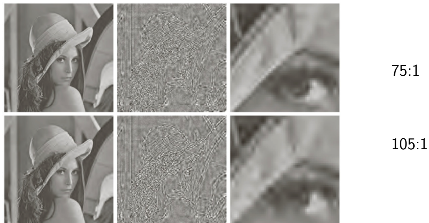
FIGURE 8.49 Four JPEG-2000 approximations of Fig. 8.9(a). Each row contains a result after compression and reconstruction, the scaled difference between the result and the original image, and a zoomed portion of the reconstructed image. (Compare the results in rows 1 and 2 with the JPEG results in Fig. 8.32.)
