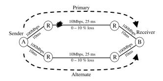
Fig. 14. Simulation network topology with random loss, equal delays, and primary path failure.
