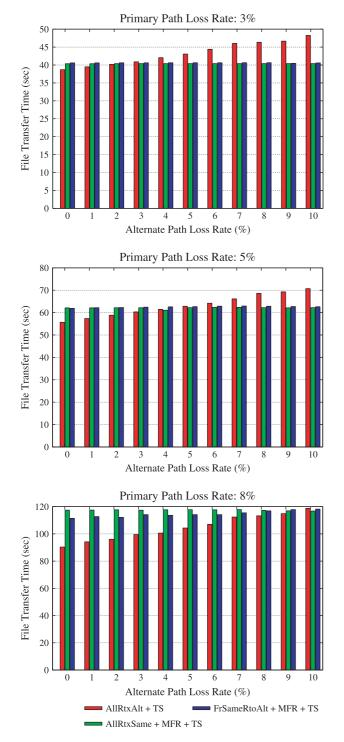
Fig. 12. AllRtxAlt+TS, AllRtxSame+MFR+TS, and FrSameRtoAlt+MFR+TS at  $\{3, 5, 8\}\%$  primary path loss, 90 ms primary path RTT, and 90 ms alternate path RTT.
