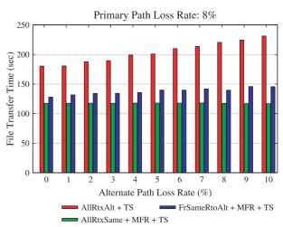
Fig. 13. AllRtxAlt+TS, AllRtxSame+MFR, and FrSameRtoAlt+MFR+TS at  $\{3, 5, 8\}\%$  primary path loss, 90 ms primary path RTT, and 1040 ms alternate path RTT.
