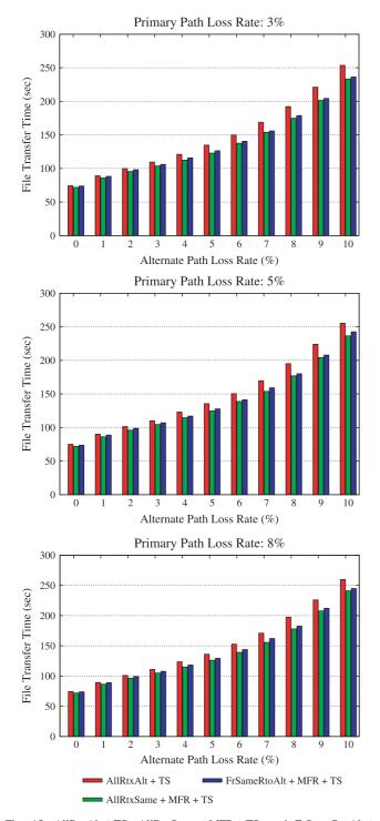
Fig. 15. AllRtxAlt+TS, AllRtxSame+MFR+TS, and FrSameRtoAlt+MFR+TS with primary path failure at time=4 s.
