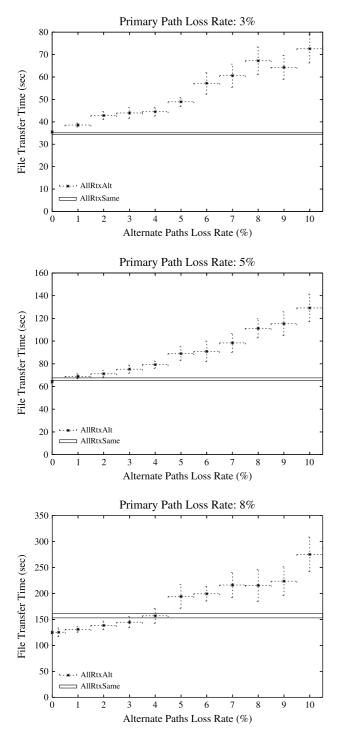
Fig. 3. AllRtxAlt vs AllRtxSame at {3, 5, 8}% primary path loss.
