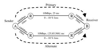
Fig. 11. Simulation network topology with random loss, 90 ms primary path RTT, and {90, 210, 1040} ms alternate path RTT.
