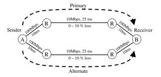
Fig. 5. Simulation network topology with random loss.
