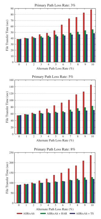
Fig. 8. AllRtxAlt and its extensions at {3, 5, 8}% primary path loss.
