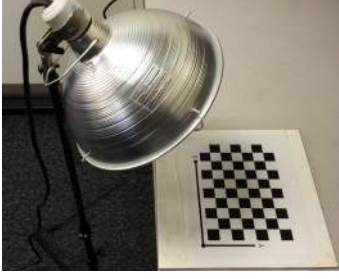
Fig. 1. Our setup includes a printed paper calibration pattern, a glazed finish ceramic tile backing to keep the pattern flat and retain heat, and a 250W heat lamp.
