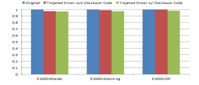
*Fig. 4:* Comparison of normalized CPU performance among original driver, driver infected by rootkit without the checksum code, and driver infected by rootkit with the checksum code
