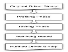
Fig. 1: Overview of kernel driver purification
