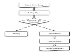
Fig. 6: Kernel Driver Purifier with Checksum Detection
