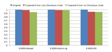
Fig. 5: Comparison of normalized network throughput among original driver, driver infected by rootkit without the checksum code, and driver infected by rootkit with the checksum code
