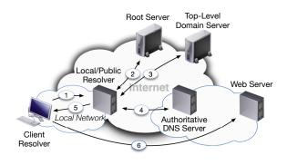
Fig. 1. DNS Resolution Process (Iterative query).
