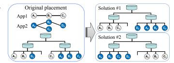
Fig. 1. An example of two equivalent solutions with different transition costs
