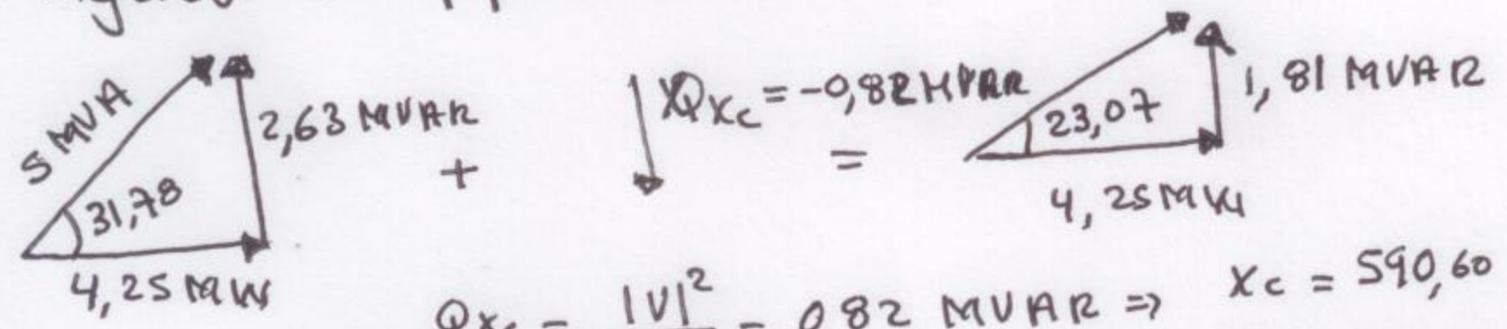
$$Q_{xc} = \frac{VI^2}{X_c} = 0,82 \text{ MVAR} \Rightarrow X_c = 590,60 \text{ k}\Omega \Rightarrow$$
