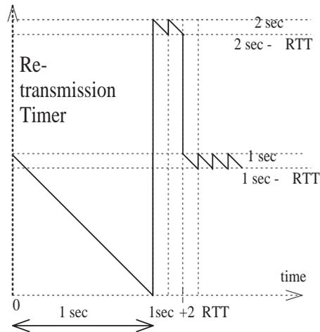
Figure 1: Behavior of the TCP retransmission timer
