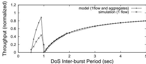
Figure 4: DoS TCP throughput: model and simulation
