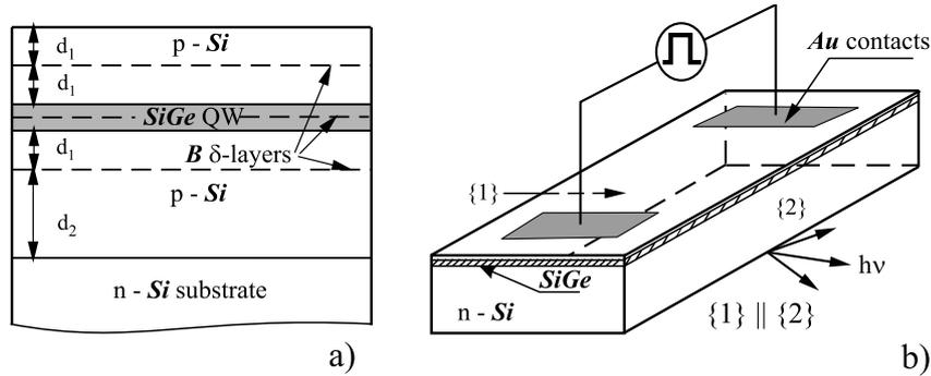
**Fig. 1** Schematic view of structure (a) and laser design (b).
