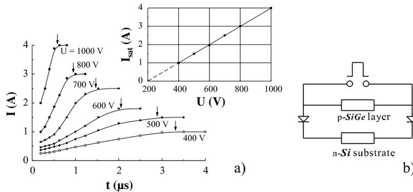
**Fig. 3** a) Current vs. time during thermal breakdown of the substrate. Arrows show the onset of stimulated emission. Inset: voltage dependence of saturation current. b) Equivalent circuit of SiGe/Si structure.
