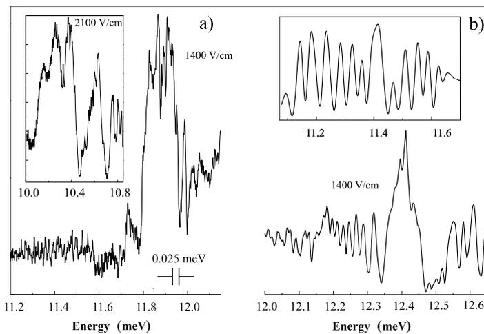
**Fig. 2** Spectra of stimulated THz emission in structures of type I (a) and type II (b) at 1400 V/cm. Insets: a) additional lines arisen in the spectrum at 2100 V/cm, b) modal structure.
