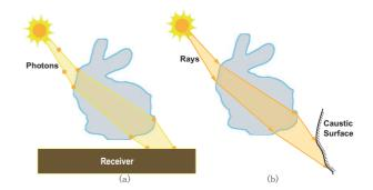
Figure 2. Caustics can be interpreted from one of two perspectives: (a) in terms of photons gathered on scene geometry, or (b) in terms of the caustic surfaces formed by light rays.
