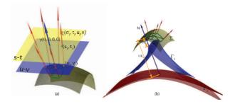
Figure 7. Surface normals can be represented as rays. (a) We orient the local frame to align the uv plane with the surface tangent plane. The neighboring normal rays can be parameterized as the intersections of the two planes as  $[\sigma, \tau, u, v]$ . (b) A smooth surface  $\Sigma$  has two sheets of normal ray caustic surfaces  $\Gamma_1$  and  $\Gamma_2$ , each formed as the loci of the corresponding loci of principal curvature's radii.
