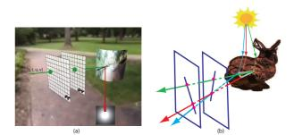
Figure 4. (a) At each point on the surface, the reflected (refracted) light ray is mapped into the ray space by intersecting with the two parametrization planes. (b) The neighboring ray triplets are constrained to pass simultaneously through two slits, which are parallel to the specified parametrization planes and rule the caustic surfaces.
