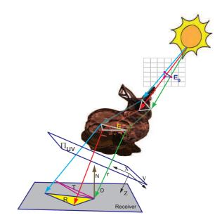
Figure 5. To compute the intensity for each ray (green), we map the neighboring ray triplet into the ray space under 2PP. We then use the ray characteristic equation to approximate the energy flex on the receiver.
