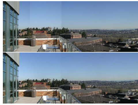
Figure 8. The image mosaic on top exhibits obvious vignetting effects. Below, the same sequence after vignetting is corrected separately in each image using our method. No image blending has been applied.
