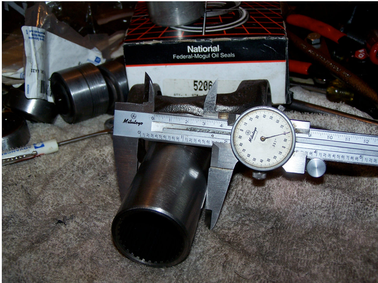
Figure 16: TH400 slip-yoke machined to Viper OD (shown with viper bushing&seal kit in background)
