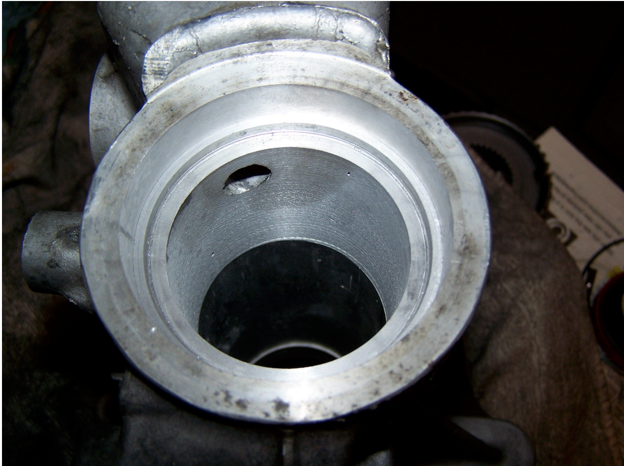
Figure 15: F-body tail housing machined for SSR bushing & seal
