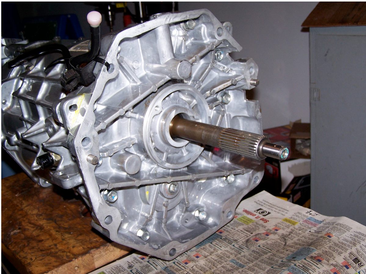
Figure 22: LS1 F-body Front Plate with C6 input shaft
