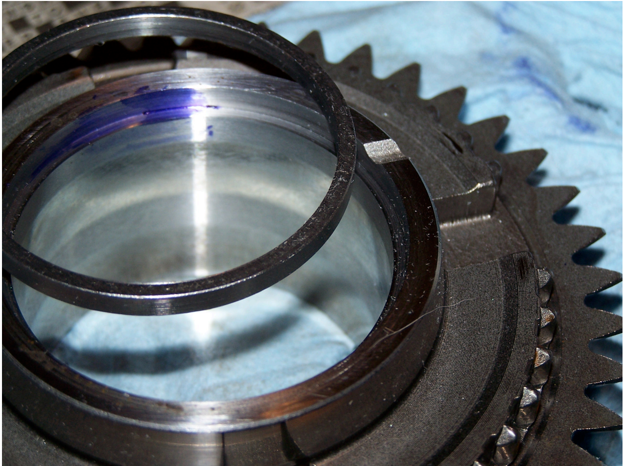
Figure 17: First Gear machined ID lip for lock retaining ring clearance
