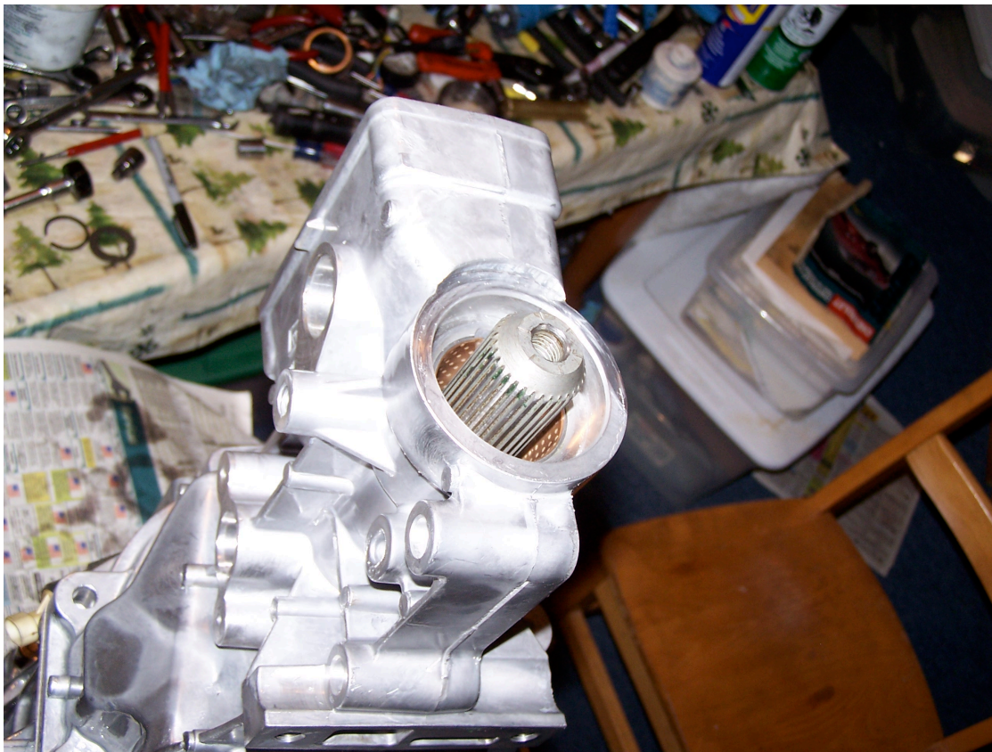
Figure 8: Factory SSR Bushing and Seal area
