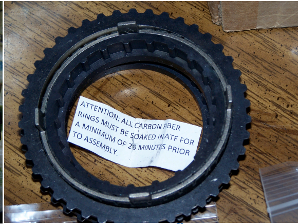
Figure 3: Older Double Cone 1 st gear Synchro blocker
