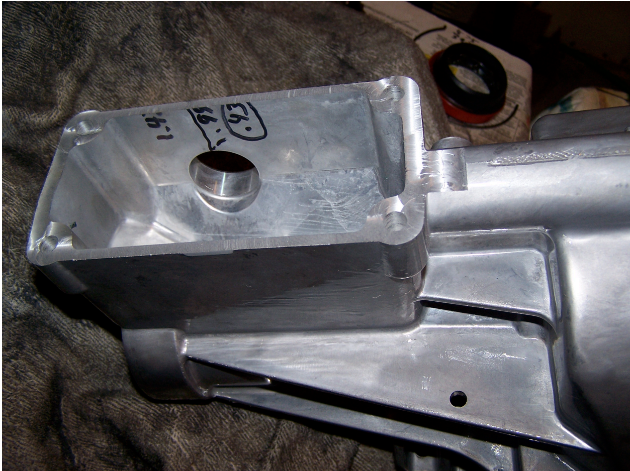
Figure 14: Machined shifter pad (0.430") of SSR tail housing
