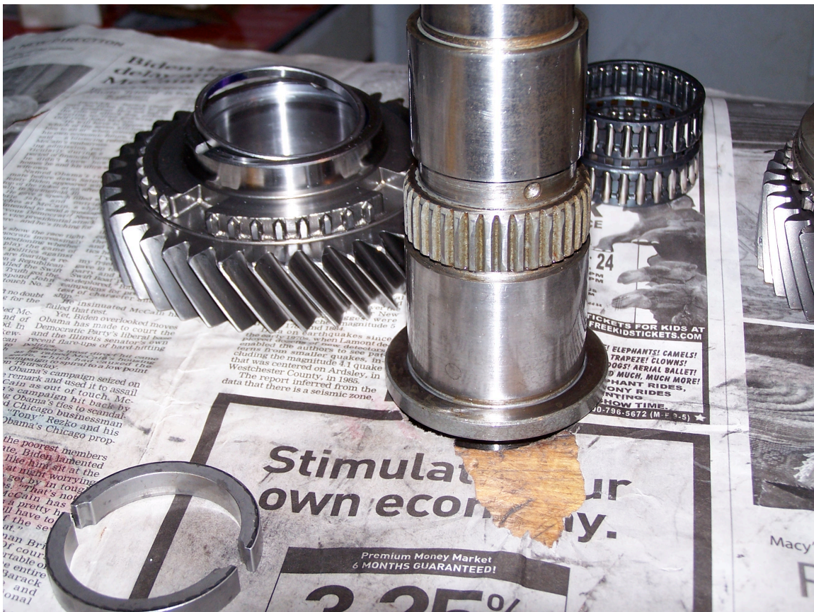
Figure 19: SSR main shaft 1-2 synchro lock retaining slot
