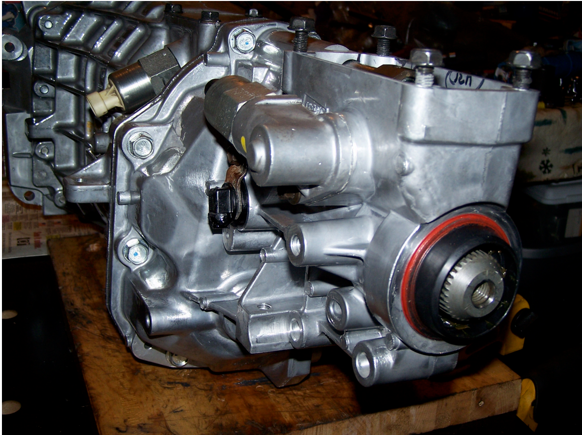
Figure 21: Completed SSR Tail housing assembled
