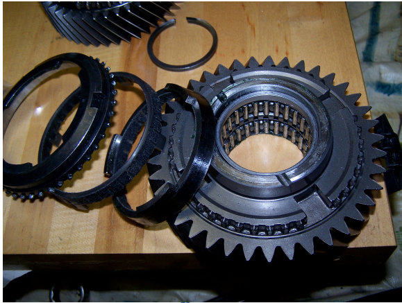
Figure 2: Triple Cone 1 st gear Synchro blocker
