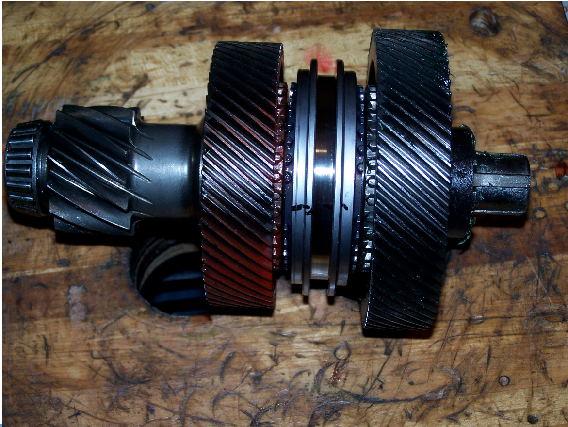
Figure 10: 2pc Extension shaft with Tapered Bearing
