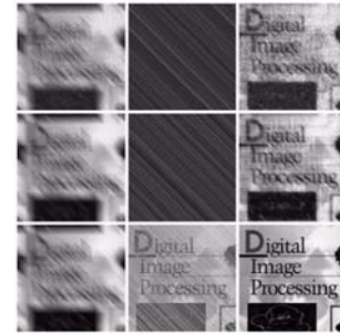
FIGURE 5.29 (a) Image corrupted by motion blur and additive noise. (b) Result of inverse filtering. (c) Result of Wiener filtering. (d) Full inverse filter result with noise variance and color of magnitude zero. (e) Same sequence, but noise variance reduced by five orders of magnitude from (c). Note in (b) how the deblurred image is quite unlike the original image.
