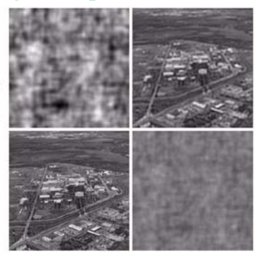
FIGURE 5.27 Restoring Fig. 5.25(b) with Eq. (5.7-1). (a) Result of using the full filter. (b) Result with H cut off outside a radius of 40. (c) outside a radius of 70. (d) outside a radius of 85.
