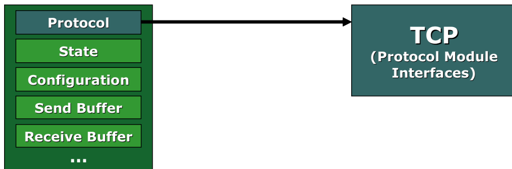
Figure 2.1: Normal TCP socket format
