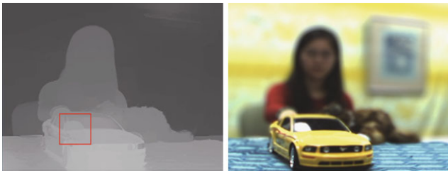
Fig. 15 Observed artifacts ( high lighted with red rectangle ) at specular regions on a computed disparity map
