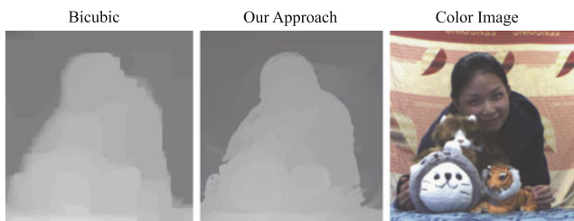
Fig. 7 Comparison between our method and bicubic upsampling on real scenes. The disparity map is upsampled from 320 \times 240 to 640 \times 480 . Our method preserves sharp edges and maintains smoothness, which is critical to reliable DoF synthesis
